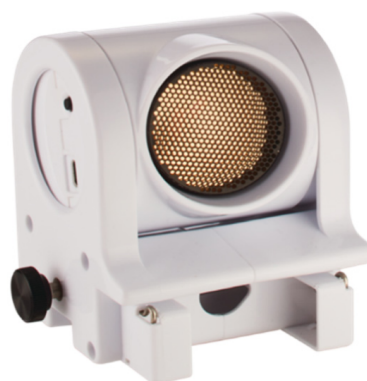
figure 2a – Wireless motion sensor PS-3219. It is small (8x8 cm) light, and easy to mount
