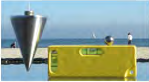
Fig. 04a. The geoid surface is defined by sea level; it is always perpendicular to the gravity force, as measured by plumb-line (beach of Sopot on the photo).
