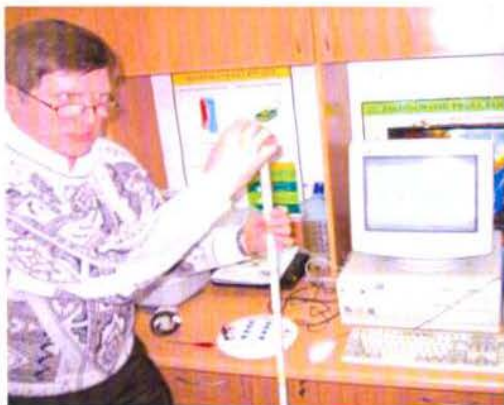
Fig. 15. Tadeusz Kubiak presents checking the dependence of magnetic induction on intensity of current flowing in the coil.
