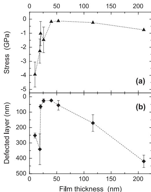
Fig. 4. (a) Compressive stress of the films and (b) depth of the defected layer in the Si substrate, as a function of the film thickness.
