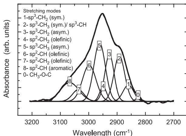
Fig. 1. A typical C–H stretch absorption spectrum for the films under study.
