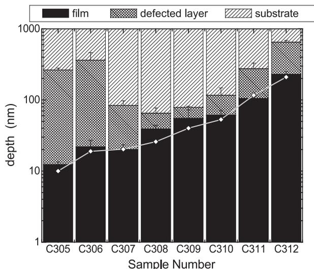
Fig. 3. Layered structure of the  $a$ -C:H films as obtained by fitting the PAS measurements. First layer: carbon film, second layer: defected layer of the Si substrate, third layer: undefected Si substrate. The white diamonds indicate the thickness of the films as measured with profilometer.
