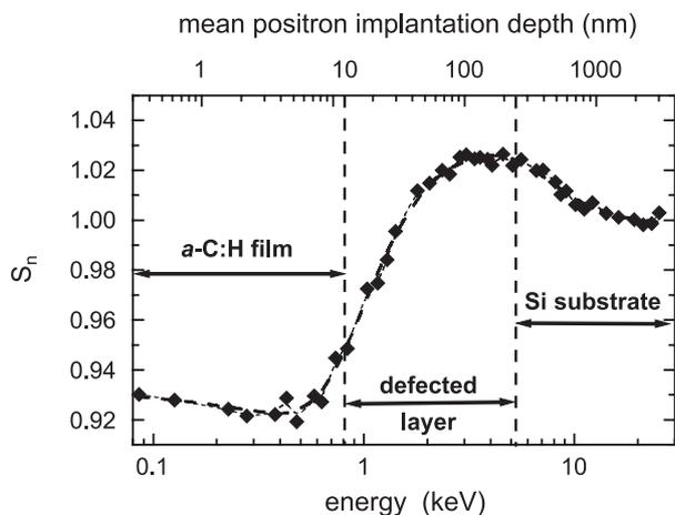
Fig. 2. Positron annihilation with low momentum electrons ( $S_n$ ) versus positron implantation energy for the 11-nm-thick film. The mean positron implantation depth is reported on the upper scale.
