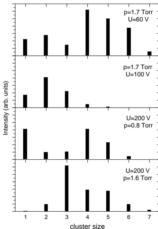
Fig. 2. Present mass spectra obtained for different experimental conditions.
