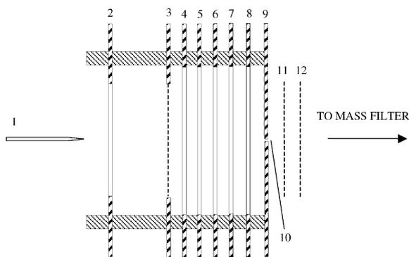
Fig. 1. Diagram of ion source and drift cell: 1 and 2, ion source; 3, tungsten grid; 4–9, guard electrodes; 3–9, drift region; 10, pinhole; 11 and 12, grids.
