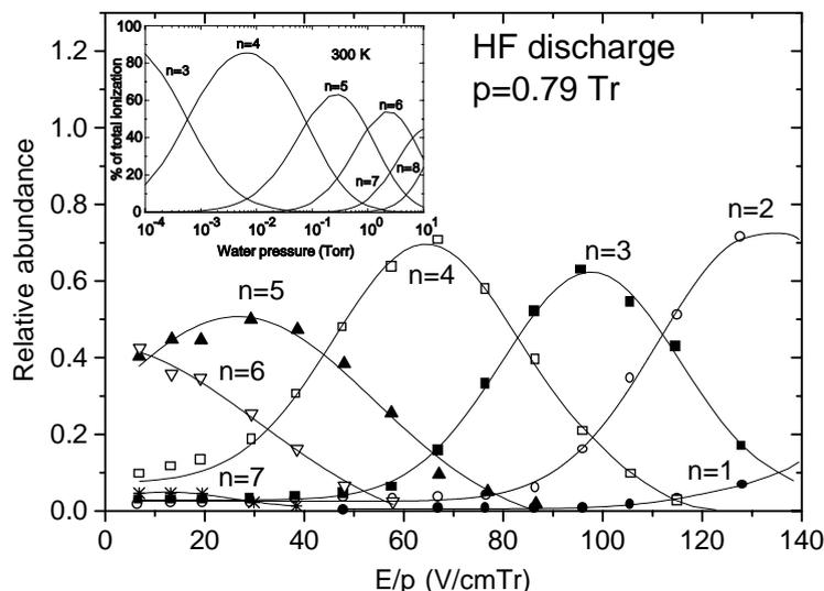
Fig. 3. Dependence of cluster population for alternate current HF discharge at variable ratio of electric field to pressure at constant pressure in the drift chamber. On insert thermodynamical results of Kebarle et al. (1967) are shown.
