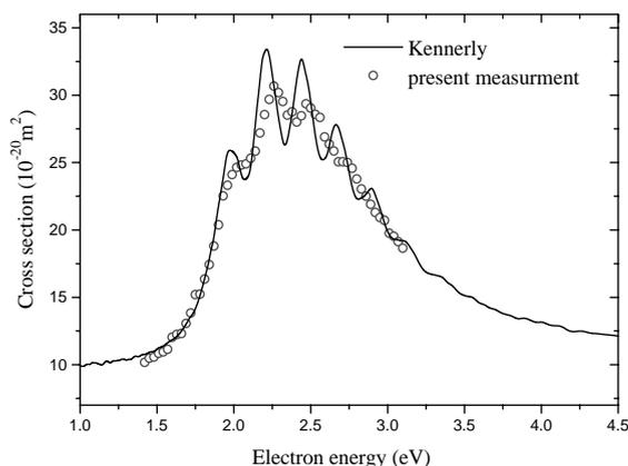
Fig. 4. Total cross section for electron scattering on  $N_2$ : the present measurements are compared with the data of Kennerly (1980). This measurement allows to determine the apparatus energy resolution as  $(\Delta E/E \sim 130/2 \text{ meV/eV})$ .
