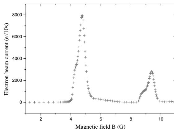
Fig. 2. Apparatus transmission function as measured with an electron beam. The presence of the peaks is determined by the focussing properties of the axial magnetic field.
