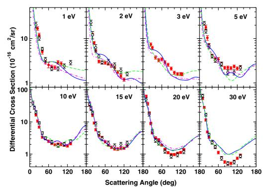
FIG. 3. (Color online) Comparison of present measured DCSs for elastic electron scattering by isobutanol with earlier results. Filled red circles are present isobutanol measurements; open circles are *n*-butanol measurements of Ref. [8]; solid blue line is the isobutanol calculation of Ref. [4]; dashed green line is the pseudopotential calculation for *n*-butanol of Ref. [8]; and chained magenta line is the present calculated result for isobutylamine.
