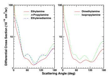
FIG. 5. (Color online) Calculated differential cross sections at 10-eV impact energy for elastic electron scattering by five small alkyl amines. The molecules in the left panel show primarily an f-wave pattern, with a minimum at  $90^{\circ}$  flanked by two local maxima or shoulders; the molecules in the right panel show an approximate d-wave pattern, with a local maximum near  $90^{\circ}$ .
