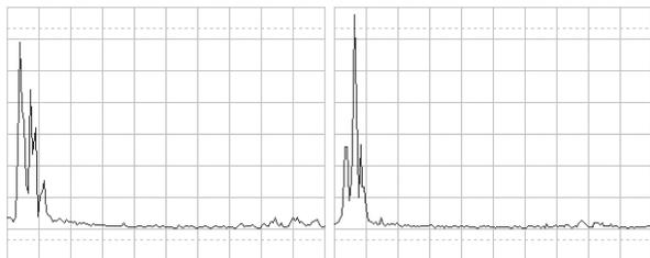
Fig. 10. Reverberation effects on the big thunder tube – intensities of different frequencies fall and grow in time. Single pictures of the presented Fourier-analysis sequence were taken every 0.2 s.
