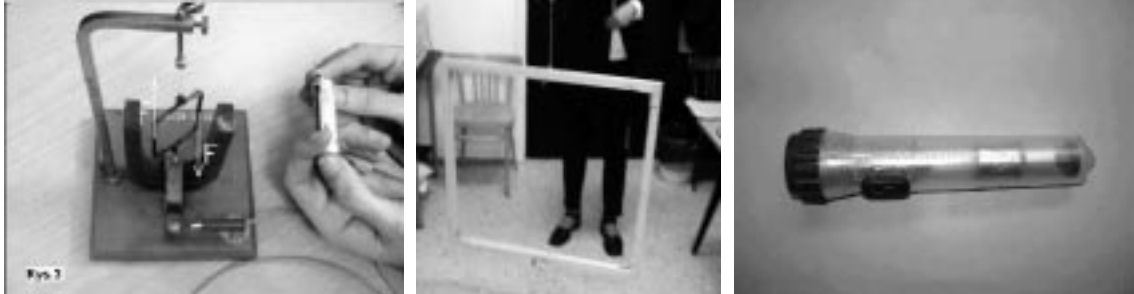
Fig. 3. AC current sources, or electric motors: a) a turning coil from the school lab [5], b) Helmholtz's coil - about 100 windings of 0.8 mm diameter wire (the chair and Ania's legs in the background are not necessary) c) hand-shaken lamp – the current is generated moving a magnets incite the coil (made in China).
