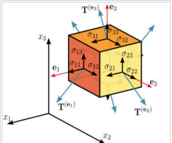
Figure 2.3 Components of stress in three dimensions
