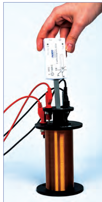
Wirelessly measure the magnetic field strength inside a solenoid as a function of current.
