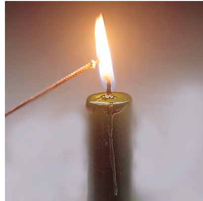
The Type K Temperature Sensor can be used to measure the temperature of a flame. Works with any industry standard Type K thermocouple.
