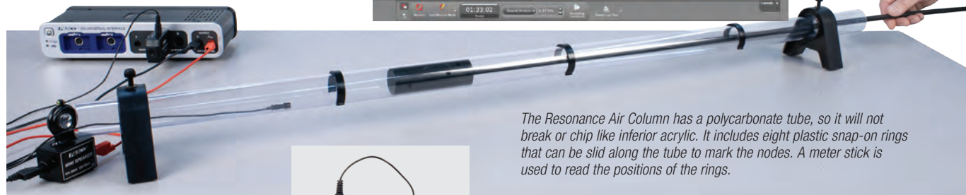
The Sound Sensor (UI-5101) has a microphone on a 1.4 m long wire, so it can be used to find the nodes inside the Resonance Air Column.
