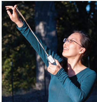
The Wireless 3-Axis Acceleration/Altimeter is launched by a stretched rubber band that is connected to one of the many attachment holes in the rubberized case. The graph shows the resultant acceleration (measured in g's) and the altitude for the four-second flight.
