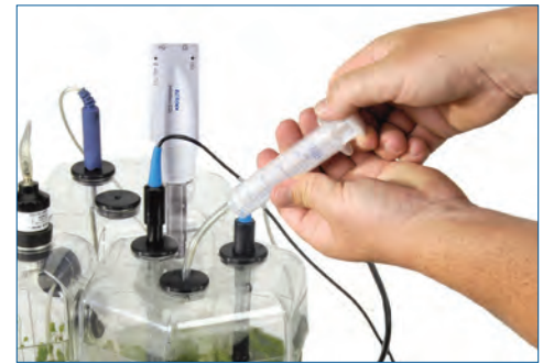
Keep the system closed during chemical testing. Use the included syringe to extract water, or inject pollutants into the system and see how the ecosystem responds.
