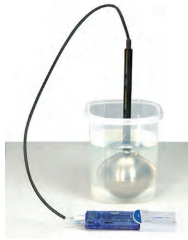
Measure the pressure and temperature of air in the sphere.
