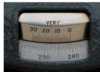
The Vernier Scale resolves angle measurements within 1 minute of arc.
