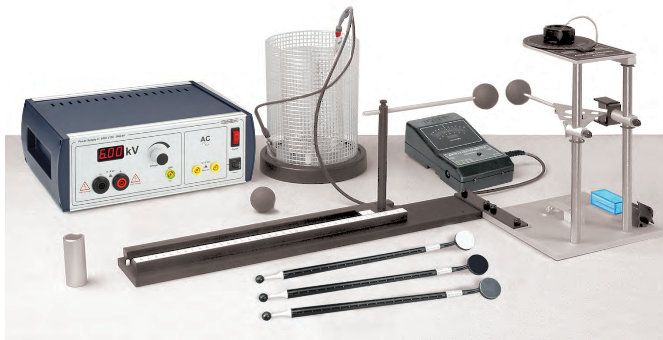
When an electrostatic force is applied, the torsion wire is twisted to return the balance to equilibrium. The twist of the wire is proportional to the electrostatic repulsion force.
