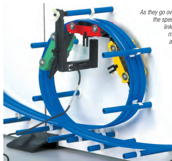
Conservation of energy shows that the final speeds of these two cars are the same even though the red car takes much less time than the yellow car to reach the end of the track.
