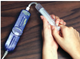
The Absolute Pressure Sensor is used in a Boyle's Law experiment in which a syringe is compressed.
