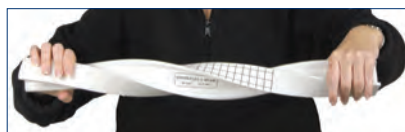
Demonstrate lack of torsional strength.
