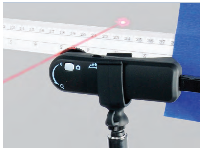
The USB Camera Microscope records the oscillation of the laser beam.
