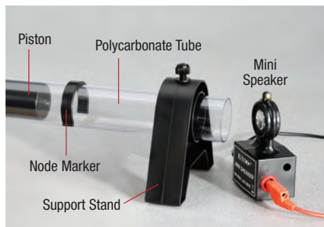
The Resonance Air Column has a polycarbonate tube, so it will not break or chip like inferior acrylic. It includes eight plastic snap-on rings that can be slid along the tube to mark the nodes. A meter stick is used to read the positions of the rings.
