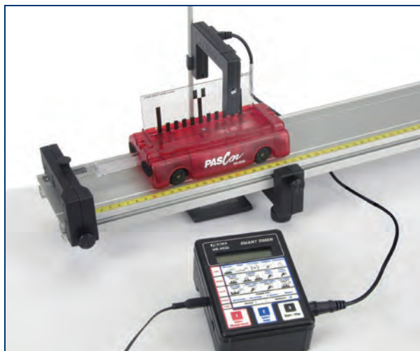
Speed of object through one gate—In Time: One Gate mode; timing begins when the photogate beam is first blocked and continues until the beam is blocked again. Use the fence supplied with the Smart Timer.
