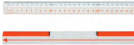
The Four-Scale Meter Stick is an important part of the Significant Figures Kit as it includes four scales of varying precision.
