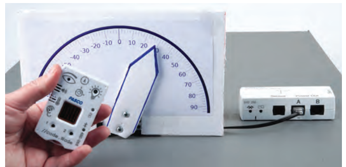
A stepper motor rotates the meter indicator to match the angle at which the //code.Node is tilted.
