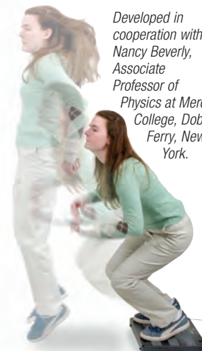
The normal and parallel forces are recorded as the girl jumps off the platform.
