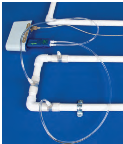
Instrument your pipe network with the Pressure Taps connected to the Dual Pressure Sensor (PS-2181).
