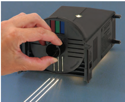
Rotate the selector knob to choose between rays (1, 3, or 5) or the primary color mask.
