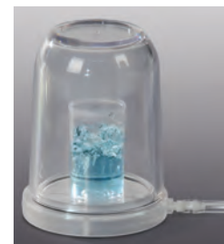
Water boils as air is evacuated from the Bell Jar.
