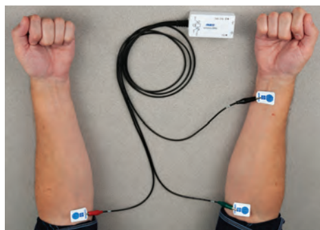
Leads on the (B) right wrist, (G) right elbow, and (R) left elbow allow the user to measure the heart's activity.
