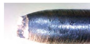
Image of broken steel tensile sample taken with the microscope.
