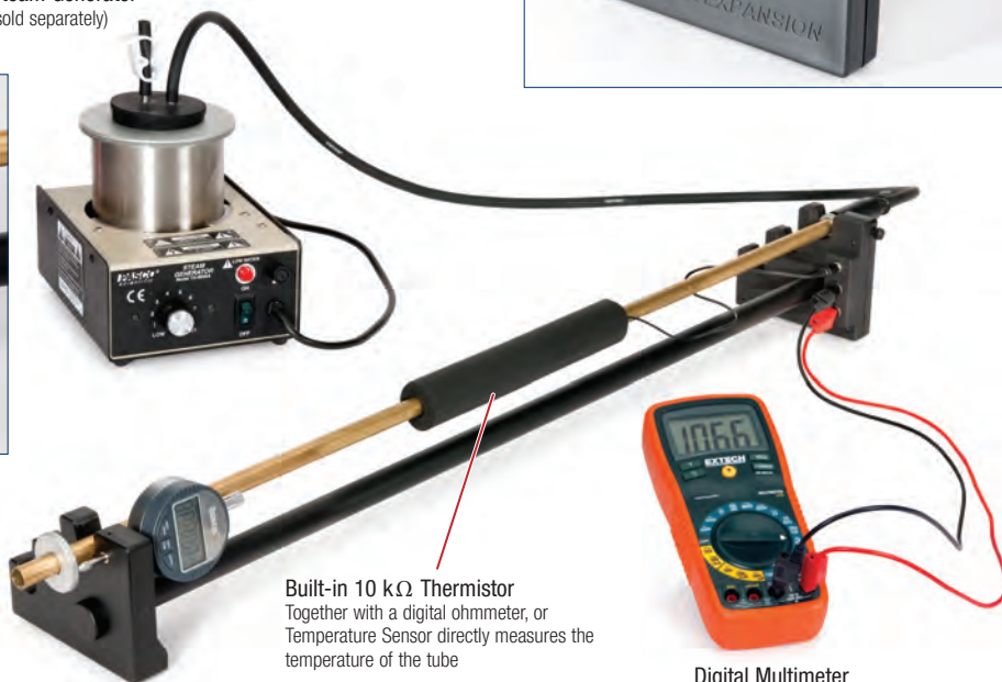
Digital Multimeter Measures thermistor resistance (sold separately)
