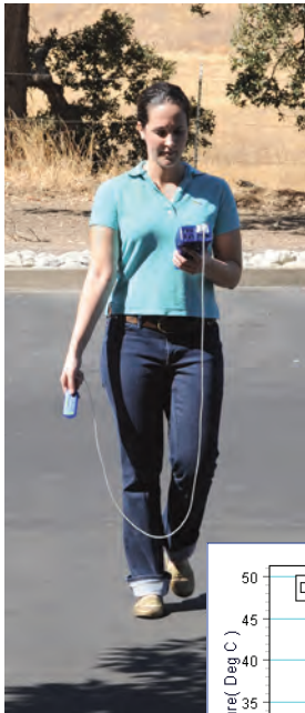
The student measures the late-morning ground temperature over four distinct surfaces. Starting in the shade under the distant tree, she then crosses bare dirt (in sun), a rock border, pavement, and lawn.
