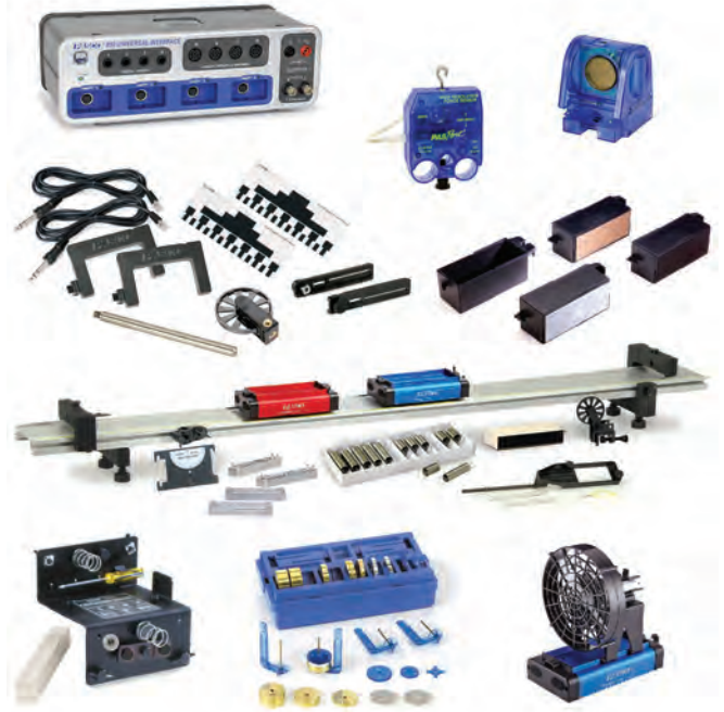
Impulse Experiment Measure the force as a function of time as the cart hits the spring and also measure the change in momentum using the photogate.
