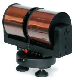
Electromagnet produces about one Tesla.
