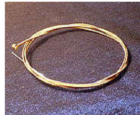
Acoustic guitar string wrapped with phosphor bronze
