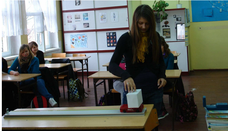
Fig. 2. Cart with box reflecting ultrasonic waves on an inclined plane. Schoolgirl takes experience during physical activities rings in Middle School No. 1 in Chelmza, which conducted the author (photo A. Karbowski).
