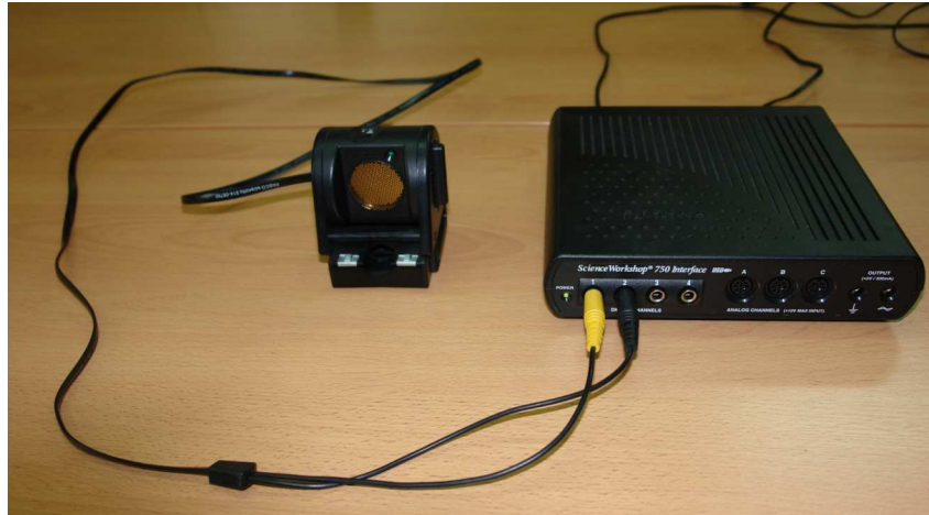
Fig. 1. The figure shows how to connect an ultrasonic position sensor Console measuring ScienceWorkshop 750.
