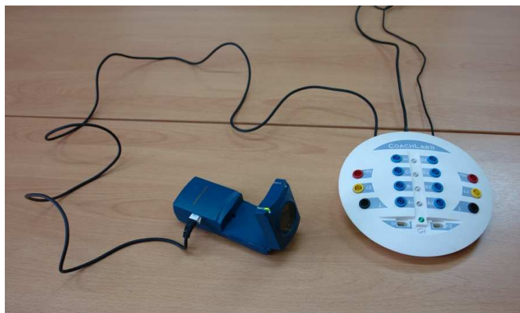
Fig. 1. The picture shows the connection of an ultrasonic distance sensor for measuring console CoachLab II (photo A. Karbowski).
