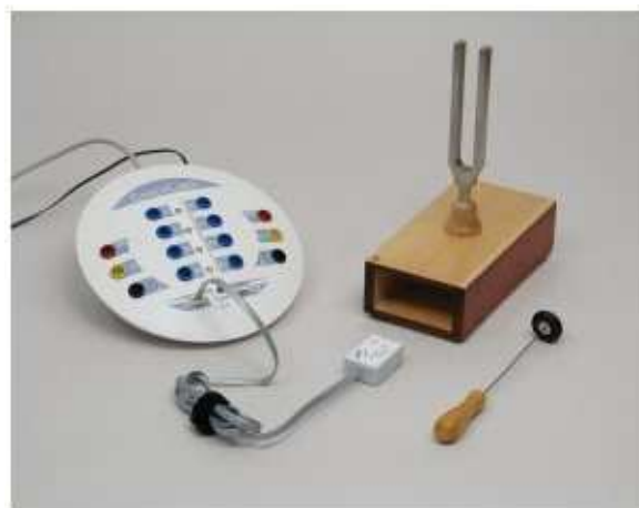
Fig.1. The figure shows how to connect to the console sound sensor measuring CoachLab II.
