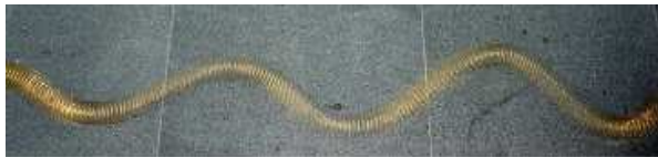
Transverse waves propagating on the spring
