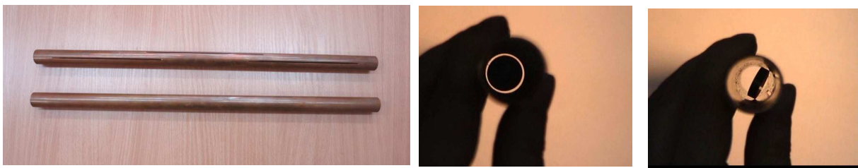
Fig. 1 Two copper tubes and magnet falling inside - general reference of the implementation in the curvilinear integral Faraday's law of electromagnetic induction. The full tube falling magnet "levitates" hanging in the air and not touching the walls; longitudinally incised in the tube falls magnet "tumbling" and bumping against the walls
