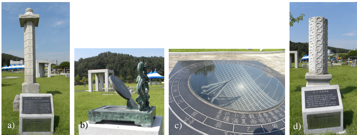
Photo 5.38. Reconstruction of historical meteo instruments and sundials in Science Museum in Daejeon: a) water-level indicator from Cheonggye river; b) reconstruction of a portable sundial from 1437 done in bronze (7-times enlarged); c) sundial Angubuilgu invented at the beginning of 15th century – extremely interesting, concave configuration of the time indicator; d) anemometer – the direction and the speed of wind was shown by a pennant at the top of the column (photo MK)
