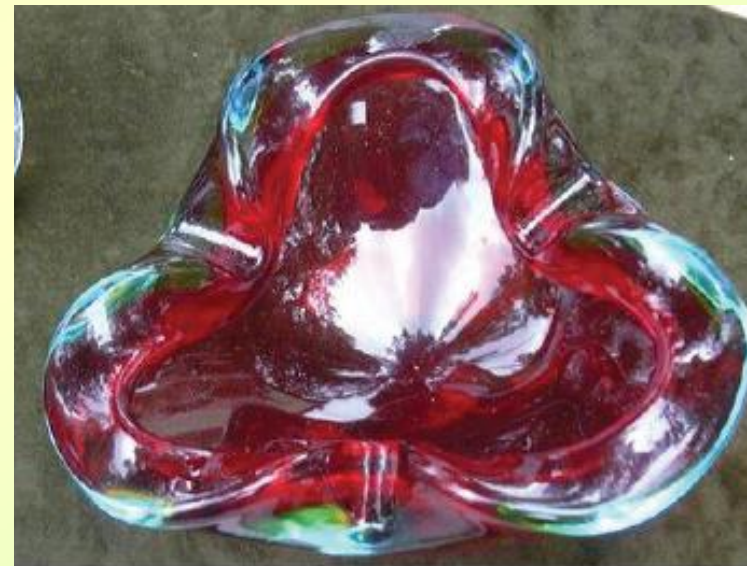
Berlin glass with Au-nanodroplets (photo GK)
