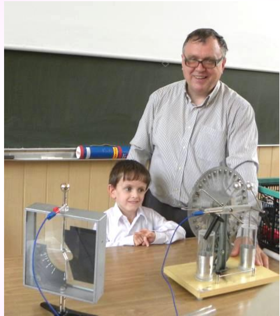
Electroscope of Volta used for measurement of the voltage from electrostatic machine.
