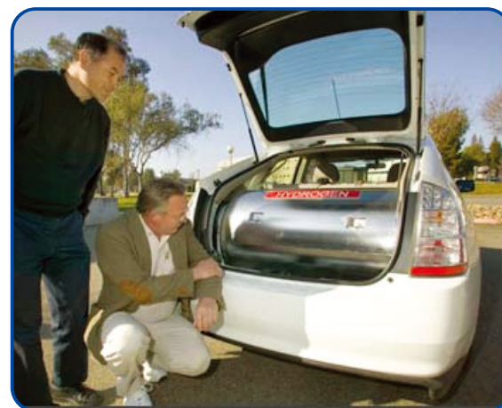
Figure 6-7. Prototype liquid hydrogen storage tank
