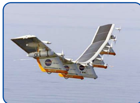
Figure 2-1. The Helios Prototype developed by AeroVironment and tested by NASA. An unmanned aerial vehicle powered by solar energy and a fuel cell system
