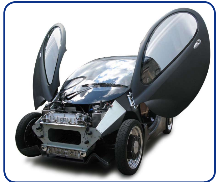
Figure 4 – Fuel Cell Car Powered by Horizon FCT Fuel Cell
