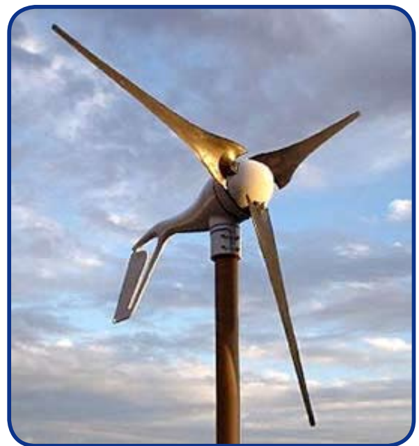
Figure 3 – Small Wind Turbine
