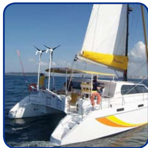
Figure 6 – Wind Turbines Charge Sailboat Batteries
