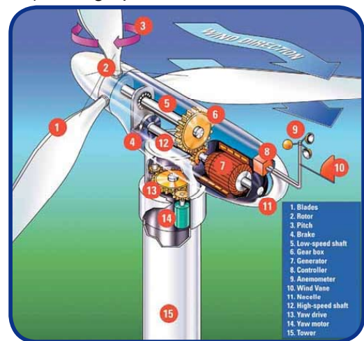
Figure 3 – Parts of a Wind Turbine
