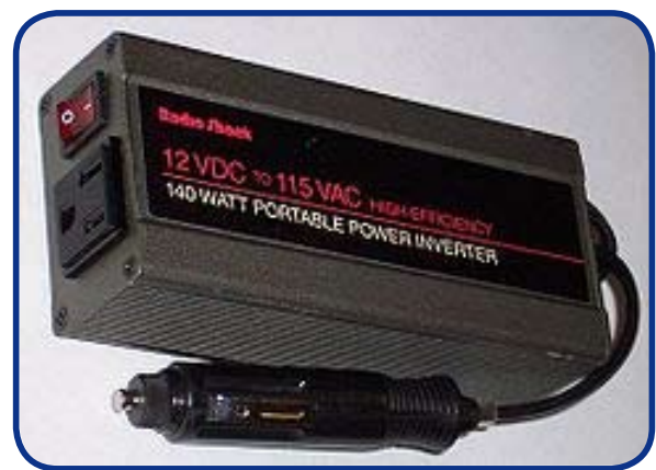
Figure 3 – Simple Appliance Inverter
