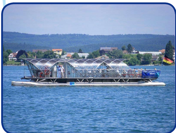
Figure 2- RA66 Helio solar-powered 20 meter catamaran
