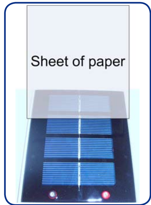
Figure 1 – Paper Shading \frac{1}{4} Solar Panel
